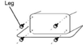
If the floor is uneven adjust the legs (do not insert pieces of wood, or any other objects under the legs)
